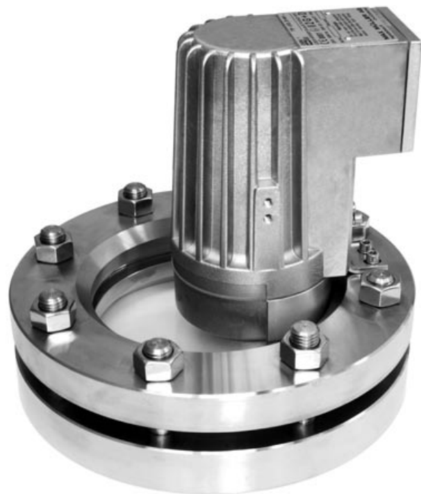
Type HEL 50 deHW, Ex de IIC T3, Ex tD A21 IP65 T195°C, Ex II 2 G + D, 230 V, 50 W, halogen version, mounted on circular sightglass to DIN 28120, DN 125, PN 10, in 1 port version.
